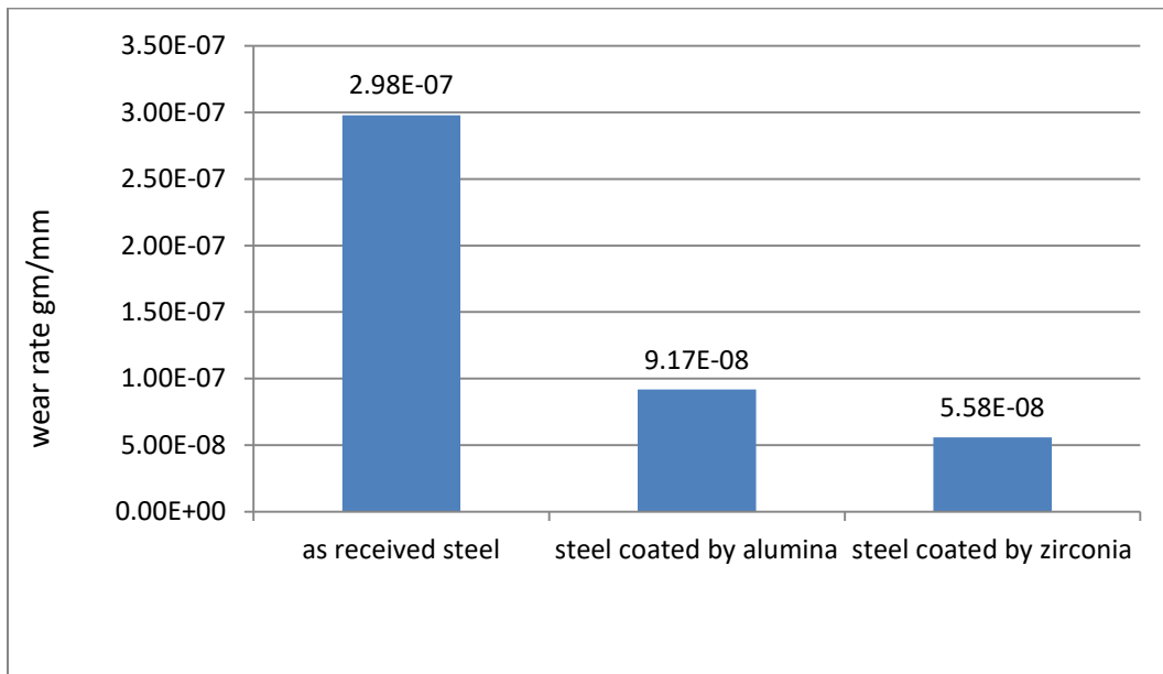
Figure.(5) Wear rates of as received steel and coating samples.
