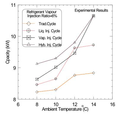
Figure (4) Effect of ambient temperatures on heating capacity.
