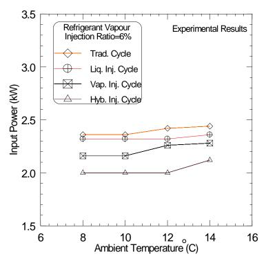
Figure (11) Effect of ambient temperatures on input power.
