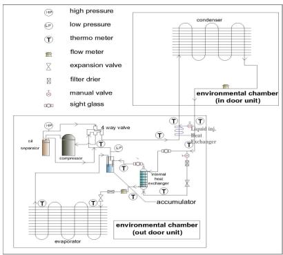
Figure (3) Experimental heat pump system.
