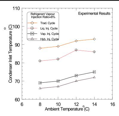
Figure (9) Effect of ambient temperatures on condenser inlet temperature.
