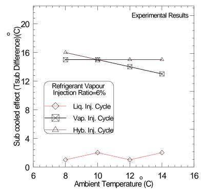
Figure (10) Effect of ambient temperatures on sub cooled effect.
