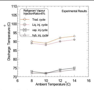
Figure (7) Effect of ambient temperatures on compressor discharge temperature.
