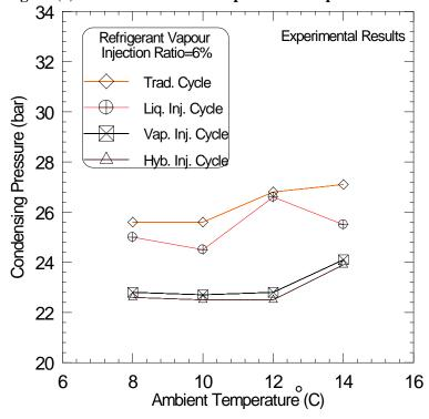
Figure (6) Effect of ambient temperatures on condensing pressure.
