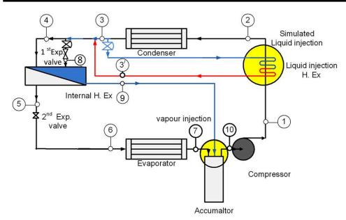
Figure (1) Schematic diagram of hybrid injection cycle.
