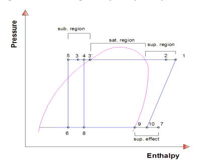
Figure (2) Pressure-enthalpy diagram for the hybrid injection cycle.
