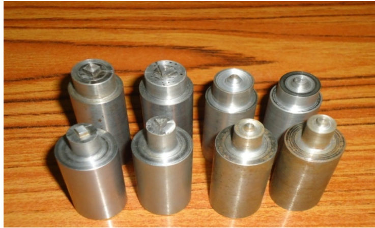
Figure 2: Image of FSW tools used in the present work
