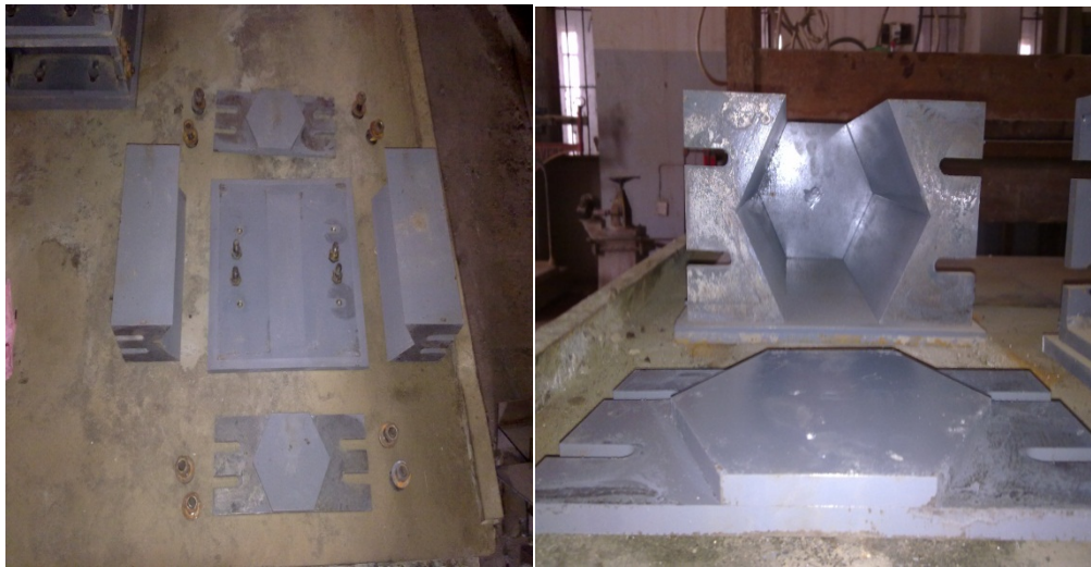
Plate 1: Mould assembly of the hexagonal specimens
