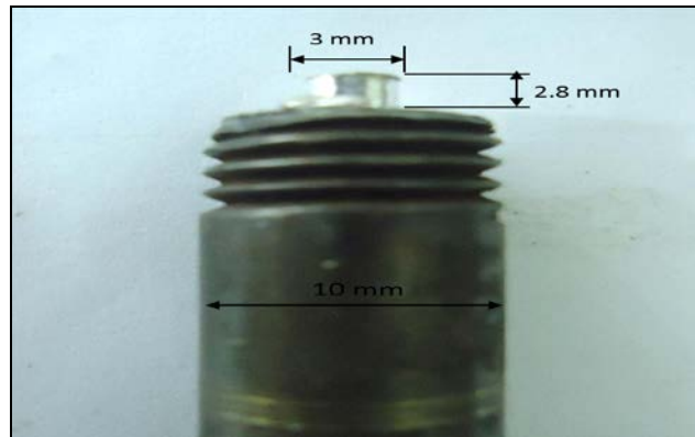
Figure (2) Tool geometry used in present work
