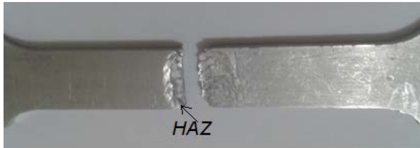
Figure (5) FSW joints failed at heat affected zone (HAZ) of the advancing side (AS)
