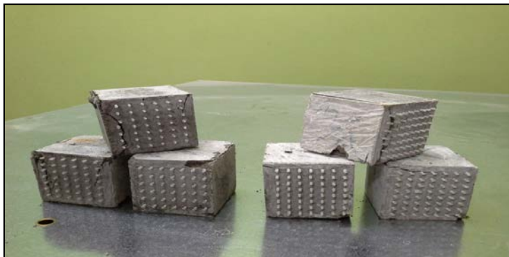
Figure (8): The specimens after compressive strength test.
