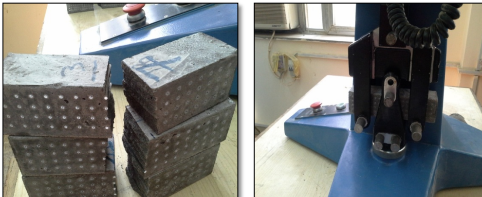
Figure (9): Flexural testing machine and test samples.
