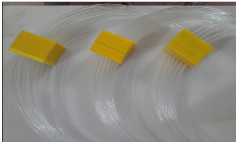
Figure (2): Details of fixing the POFs through the square plastic sheet for cubic samples.
