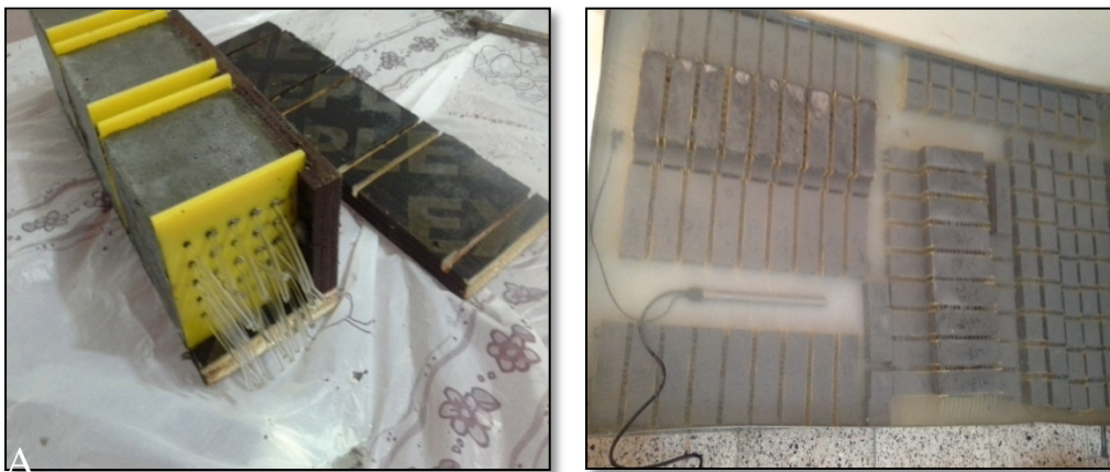
Figure (5): The specimens after de-molded and Curing of samples.
