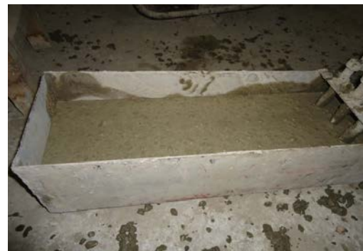
Figure (2) Flowing of concrete in horizontal section in L-box test of SCC
