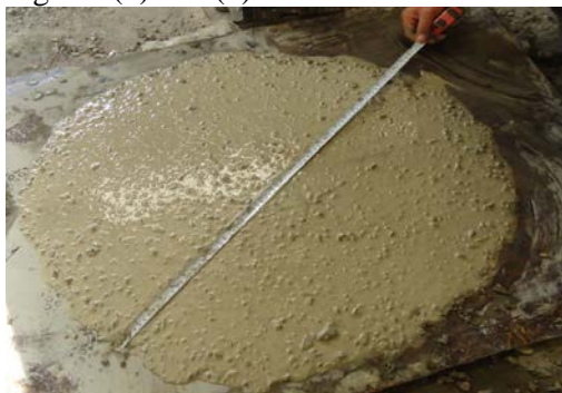
Figure (1) Spreading concrete in Slump Flow test of SCC
