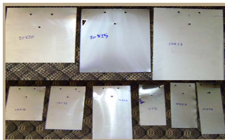
Figure (3) Nine test samples of cantilever plates
