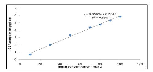
Figure(7) : Effect of initial concentration on adsorption capacity of (JGB) onto (PSC) (0.3mm particle size and 1.5gm adsorbent dose)
