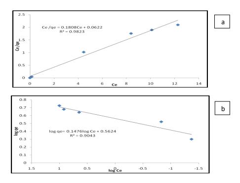
Figure(8): Linearized adsorption isotherm model of (JGB) onto (PSC)
