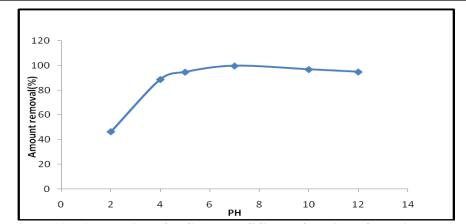
Figure(6) : Adsorption of (JGB) by (PSC) as a function of solution pH at initial concentration of 50 mg/l and adsorbent dosage of 1.5 g with 0.3mm particle size
