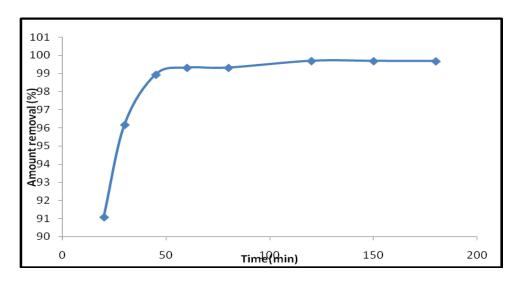
Figure (4): Effect of contact time for adsorption of (JGB) onto (PSC) at initial dye concentration of 50 mg/l, adsorbent dose of 1.5 g, and particle size of 0.3mm
