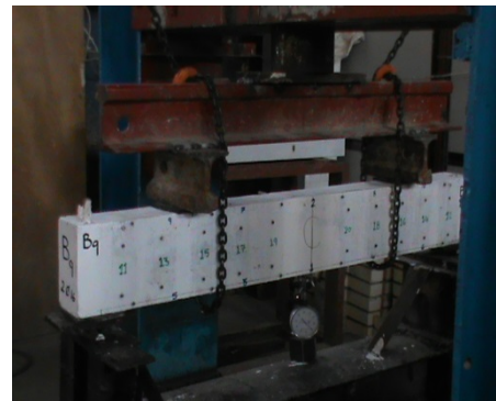
Figure (7) Beams Testing Machine Details (21)
