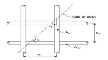
Figure 21: Calculation of web reinforcement in ACI 318-11<sup>[17]</sup>
