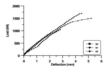
Figure (13) Load-Deflection Relationship of UHPC(hR/h=1) Deep Beams
