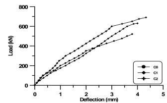
Figure (14) Load-Deflection Relationship of Hybrid Deep Beams (hR/h=0.25)
