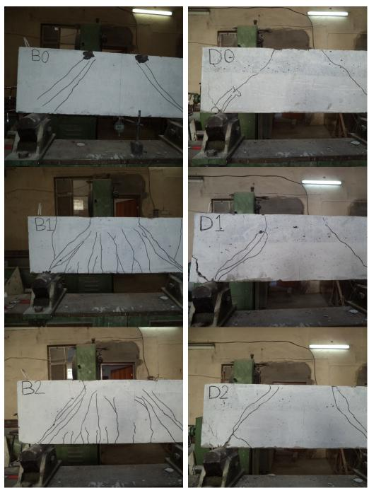
Figure (19) Beam specimens after testing to failure
