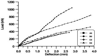
with (Vf=0%) Figure (16)Effect of UHPC layer thickness on load-deflection of Deep beams
