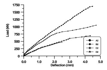
Figure (18) Effect of UHPC layer thickness on load-deflection of Deep beams with (Vf=1%)
