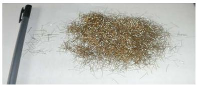
Figure (2) Sample of micro steel fibers used in present investigation
