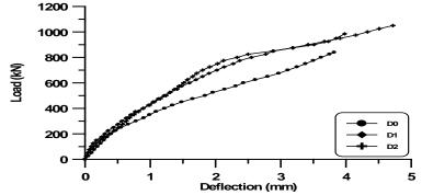
Figure (15) Load-Deflection Relationship of Hybrid Deep Beams (hR/h=0.5)
