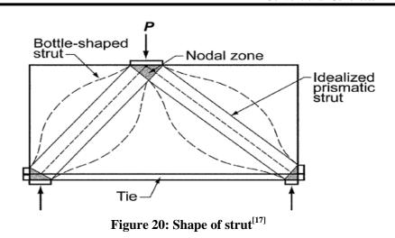
According to ACI 318-11<sup>[17]</sup> Code, the nominal compressive strength of a strut should be taken as:
