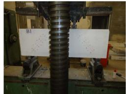
Figure (7) Deep beam inside machine
