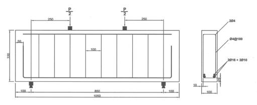
Figure (4) Typical dimensions (mm) and details of tested deep beam
