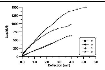
Figure (17) Effect of UHPC layer thickness on load-deflection of Deep beams with (Vf=0.5%)
