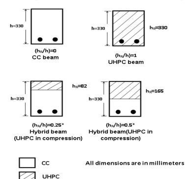
Figure (5) Types of the tested beams
