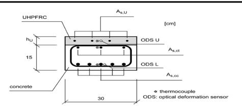
Figure (1) Cross-section of the composite "UHPFRC-concrete" beams <sup>[15]</sup>
