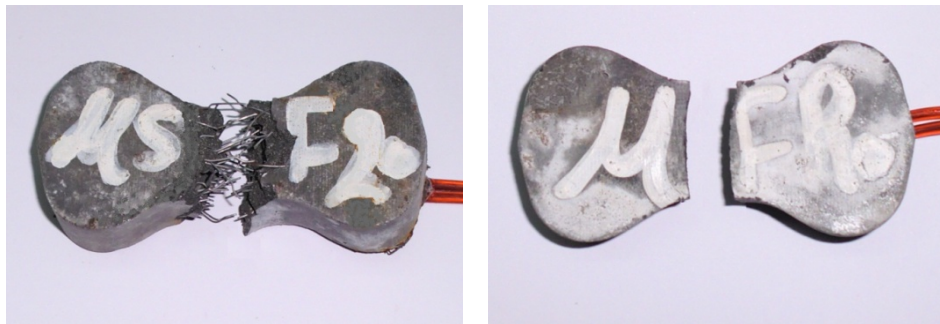
Figure (6) Tension failure of UHPC briquettes with and without steel fibers
