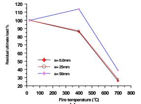
Figure (9): Effect of fire temperature on the residual load capacity of SCC column.
