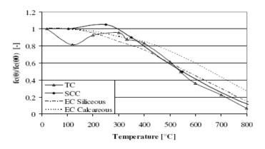
Figure (1): The residual compressive strength [8].
