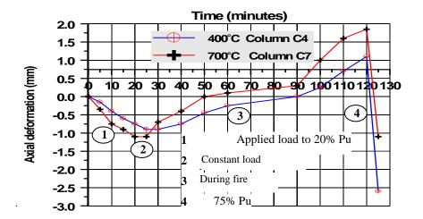
Figure (11): Axial deformation recorded at 50 mm from the centerline of column specimen before, during and after burning.
