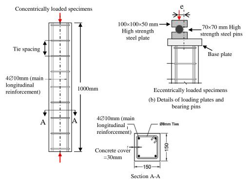
(a) Specimen dimensions and reinforcement details
