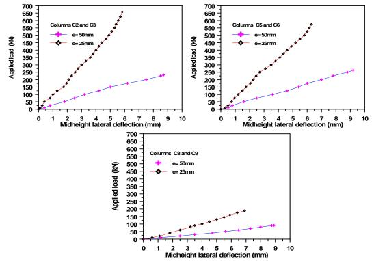
Figure (12): Comparison of eccentric load-midheight deflection curves of SCC columns.
