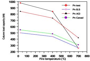
Figure (17): Effect of fire temperature on the axial load capacity of SCC column spedimens.
