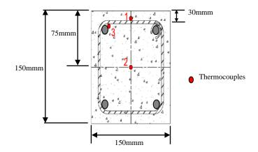
Figure (7): Thermocouples locations at midheight section in model SC columns.
