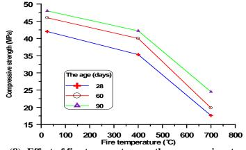
Figure (8): Effect of fire temperature on the compressive strength.
