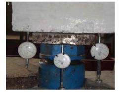
Figure (5): Testing measurement of axial deformation.
