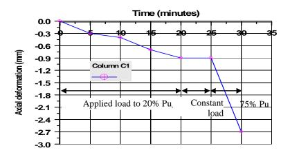
Figure (10): Axial deformation recorded at centerline of column specimen before burning.
