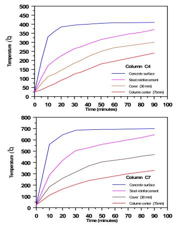
Figure (18): Temperature recorded at midheight in columns C4 and C7 as a function of time.
