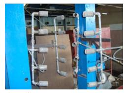
Figure (3): Network methane burners.
