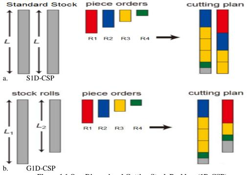
Figure 1.1 One-Dimensional Cutting Stock Problem (1D-CSP)
