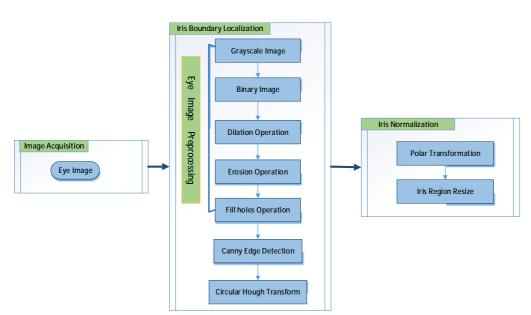
Figure (2) Block Diagram of the proposed Iris Normalization.
