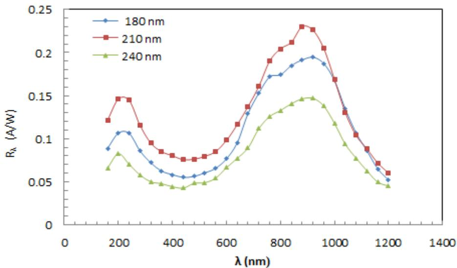
**Figure (1) Responsivity for n-Bi<sub>2</sub>O<sub>3</sub>/p-Si device fabricated at different active layers thickness.**
