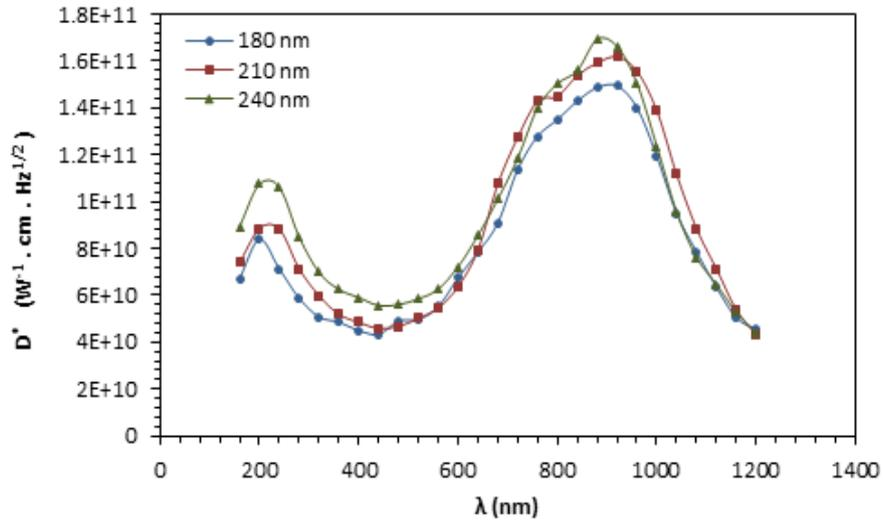
**Figure (2) Detectivity for n-Bi<sub>2</sub>O<sub>3</sub>/p-Si devices fabricated at different active layers thickness.**
