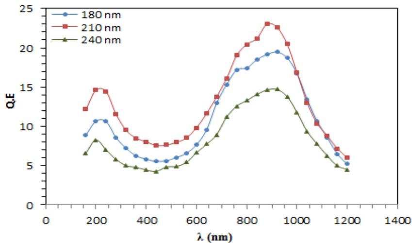
**Figure (3) Quantum efficiency for n-Bi<sub>2</sub>O<sub>3</sub>/p-Si devices Fabricated at different active layers thickness.**
