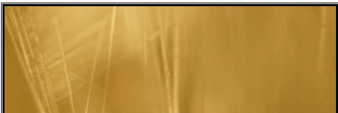
Figure (12) Optical micrograph of fracture surface for (UPE/PS , 80/20%) after the impact loading (100X).
