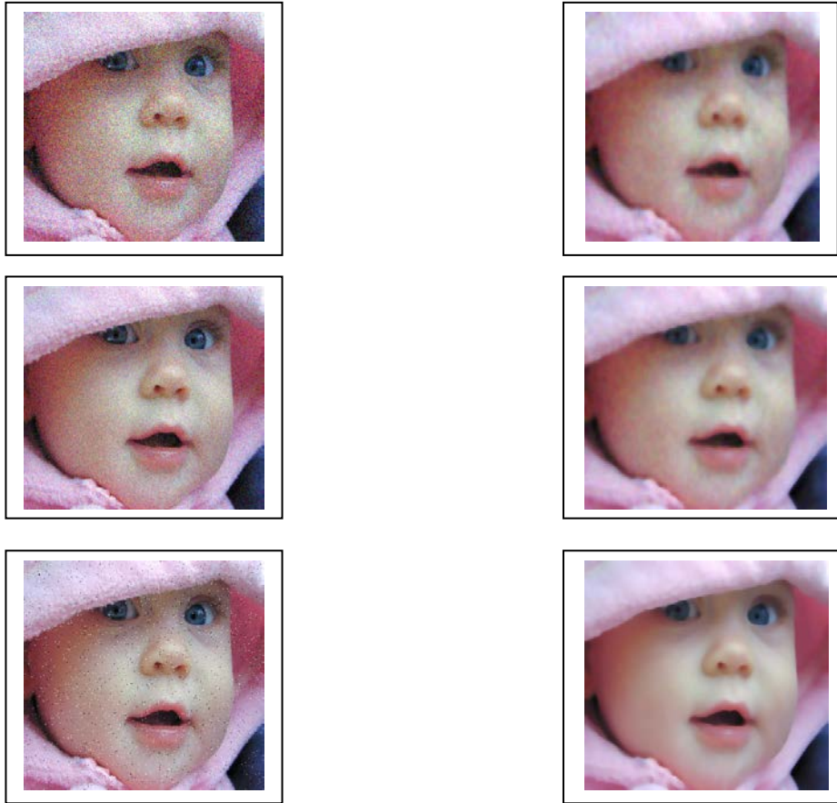
Figure (1) Left side: Images corrupted by Gaussian noise, Uniform Salt-and-pepper noise, noise ratio = 12.5 %Right side: Images after performing Median filter.
