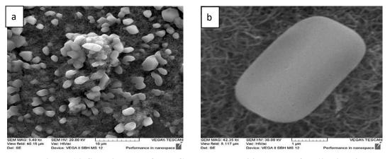
Figure (6) SEM images of MWCNTs and E.coli incubated for 60 min with normal saline prior to SEM imaging and after 8h of exposure time at different concentrations of treated-MWNTs a) 1mg,b)7mg.
