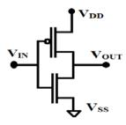
Figure (3) Structure of Nano NOT gate [12].
