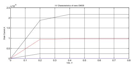
Figure (10) Current voltage characteristics for different value. of Vgs in Nano (CMOS).
