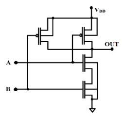
Figure (4) Structure of 2 inputs CNTFET NAND gate.
