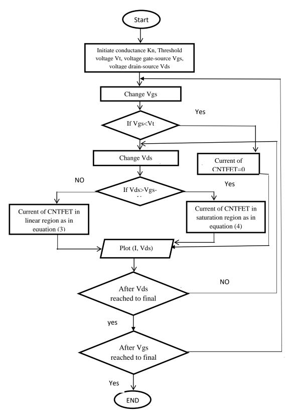
Figure (7) Flowchart of CNTFET Characteristics.
