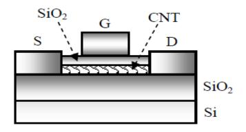
Figure (1) Schematic structures a CNTFET [10].
