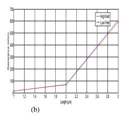
Figure (6) MATLAB results of resistance (a) length of metallic CNTs (b) Cu interconnect.
