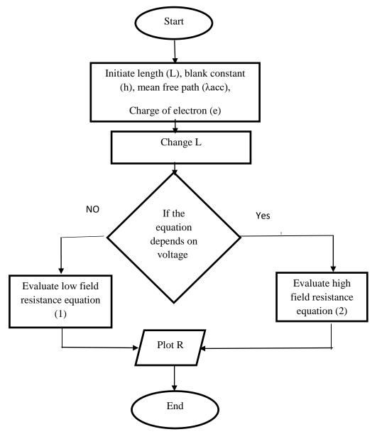
Figure (5) Flowchart of Metallic CNT Wire to simulate equation and equation (2).
