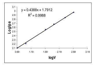
Figure (6) Plot Log Ipa(anodic current) versus Log SR(scan rate) of GPE in 0.1M KCl and 1mM K<sub>3</sub>Fe(CN)<sub>6</sub> versus Ag/AgCl.
