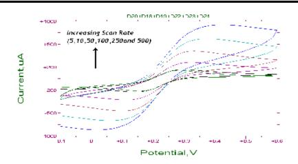
Figure (5) Cyclic Voltammetry of GPE in 0.1M KCl and 1mM K<sub>3</sub>Fe (CN)<sub>6</sub> at different scan rate (5,10, 50, 100, 250 and 500 mV sec<sup>-1</sup>) Versus Ag/AgCl and 100mVsec<sup>-1</sup>.
