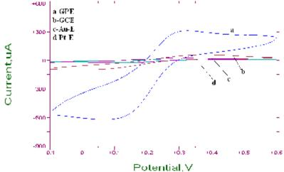
Figure (4) Cyclic Voltammetry of different electrodes (a) GPE (b)GCE (c) Au-Electrode (d) Pt-Electrode in 1mM K<sub>3</sub>Fe(CN)<sub>6</sub> with 0.1M KCl as supporting electrolyte versus Ag/AgCl and 100 mVsec<sup>-1</sup>.
