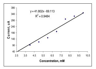
Figure (7) Plot Ipc(cathodic current) versus different concentration K<sub>3</sub>Fe (CN)<sub>6</sub> (1-10mM) in 0.1M KCl at scan rate 100mVsec<sup>-1</sup> Using GPE versus Ag/AgCl.
