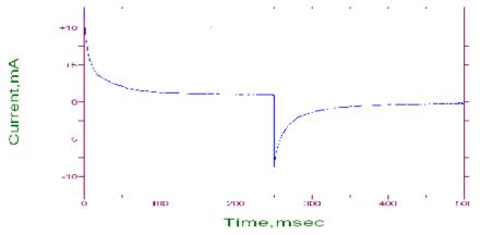
Figure (8) Chronoamperograms or Cottrell plot obtained For 1mM K<sub>3</sub>Fe (CN)<sub>6</sub> and 0.1M KCl as supporting electrolyte Using GPE versus Ag/AgCl. Potential was scanned in a negative direction from -1800 to +1800mV with 250 msec. pulse width.
