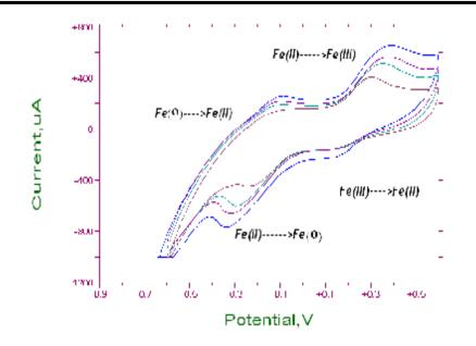
Figure (2) Cyclic Voltammetry of GPE in different concentration of 1mM K<sub>3</sub>Fe (CN)<sub>6</sub> and 0.1M KCl two redox of Fe versus Ag/AgCl and 100 mVsec<sup>-1</sup>.
