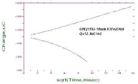
Figure (9) Choronocoulomogram or Anson plot of charge, Vs. t1/2 obtained for the redox of 1mM K<sub>3</sub>Fe(CN)<sub>6</sub> and 0.1M KCl as supporting electrolyte using GPE versus Ag/AgCl.
