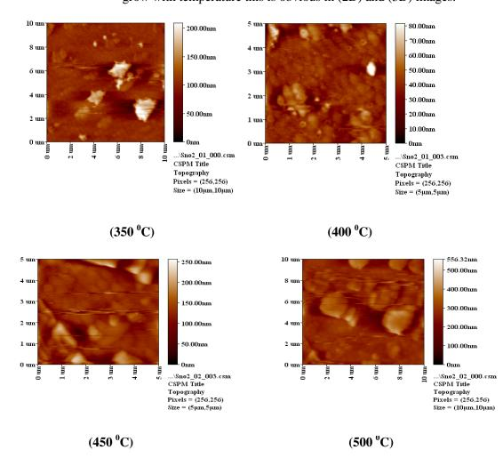
Figure (7)Atomic force microscopy(AFM) of Sno2 thin films deposit by (HPCVD in (2D).
