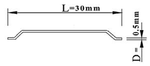
Figure (1): Sika Fiber end hooked steel fibers.
