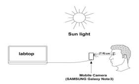
Figure (3): Proposed iris image acquisition device for real database.
