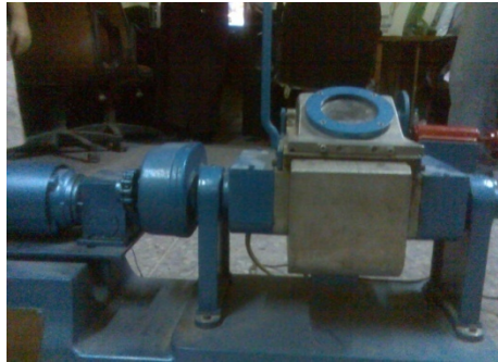
Picture(2). Shows the laboratory kneading used in forming of composite.
