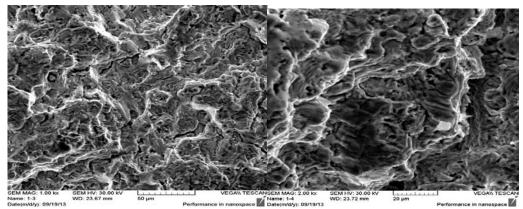
Figure (3) shows a typical ductile fatigue fracture micrograph for steel alloy CK35
