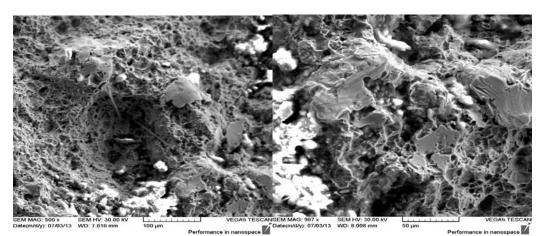
Figure (4): show micrograph of fracture surface morphology of the specimen surfaces of the pre corrosion-fatigue test for steel alloy CK35.
