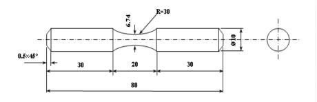
Figure (1): Specimen geometry and dimensions for fatigue test (all dimensions in mm)
