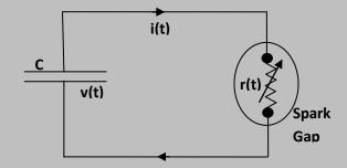
Figure (2) A schematic representation of a capacitor discharge through a time variable resistance of a spark gap.
