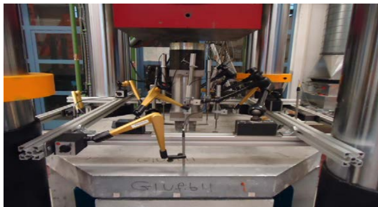
Figurer(3): Slab under test
