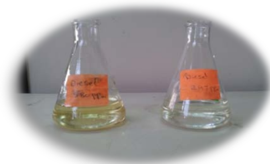
Figure (14): Left (Original Diesel Fuel); Right (Treated Diesel Fuel)
