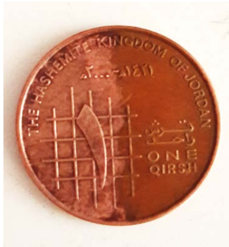
Figure (4): Laser cleaning of Jordanian copper coin using 4.89 \times 10^{10} \text{ W/cm}^2 , laser intensity.
