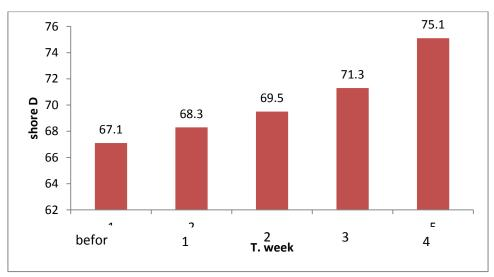
Figure (3). Shore D hardness vs. time of immersion to (optimum UP+PS)/SiO<sub>2</sub>) nanocomposite with (3% V<sub>f</sub> SiO<sub>2</sub>) before and after immersion in water
