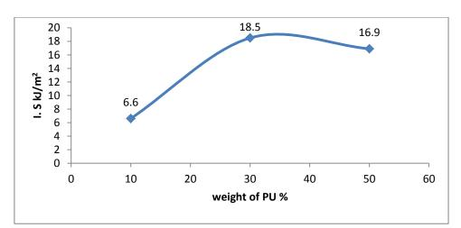
Figure (1). Impact strength of (UP/PU) blends
