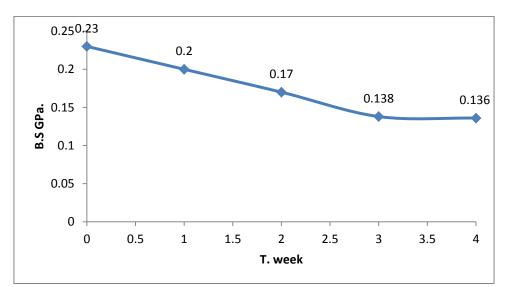
Figure (5). Change in bending strength of (optimum UP+PS)/SiO<sub>2</sub>) nanocomposite with (3% V<sub>f</sub> SiO<sub>2</sub>) before and after immersion in water
