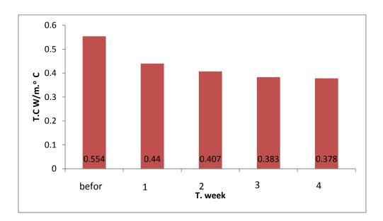
Figure (4). Change in Thermal conductivity of (optimum UP+PS)/SiO<sub>2</sub>) nanocomposite with (3% V<sub>f</sub> SiO<sub>2</sub>) before and after immersion in water
