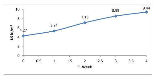
Figure(2). Impact strength of (optimum UP+PS)/SiO<sub>2</sub>) nanocomposite with (3% V<sub>f</sub> SiO<sub>2</sub>) before and after immersion in water
