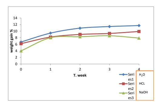
Figure(6). Change in the weight gain of (optimum UP+PS)/SiO<sub>2</sub>) nanocomposite with (3% V<sub>f</sub> SiO<sub>2</sub>) before and after immersion in different solutions.
