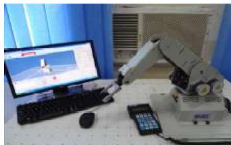
**Figure (2) 5 DOF Lab-Volt R5150 Robot manipulator systems**
