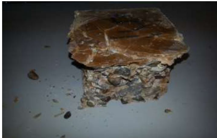
Figure (2) the polyester resin concrete specimens after compression test.
