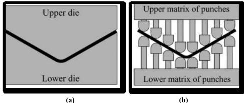
Figure (1): (a) Conventional process , and (b) MPF process [1].
