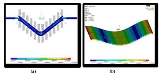
Figure (14): MPF with rubber (a) 2-D modeling, (b) 3-D modeling
