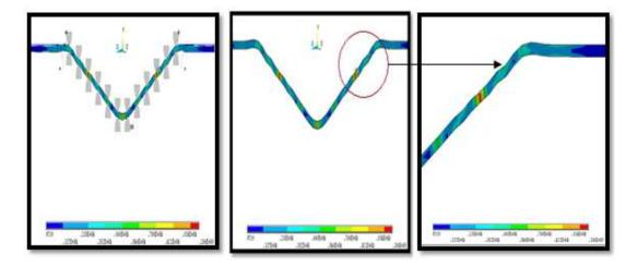
Figure (15): Final product formed by MPF without rubber
