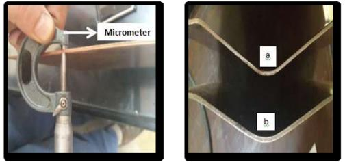
Figure (13): Thickness distribution along sheet metal formed by (a)MPF without rubber (b) MPF with rubber
