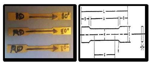
Figure (8): Rectangular cross section tensile test specimen, ASTM E8-M.[7]
