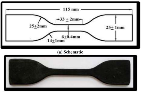
(b)Photograph Figure (9): Tensile Specimen for rubber [8]
