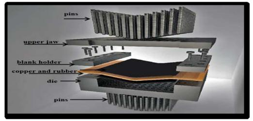
Figure (6): MPF die and pins design
