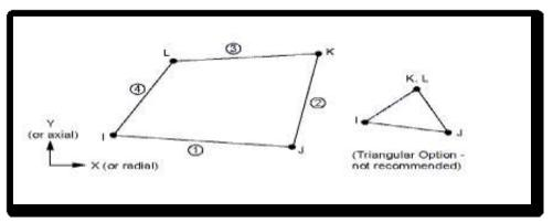
Figure (4): Element 182 geometry
