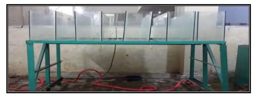
Figure (2): Containers to measure water from outlets
