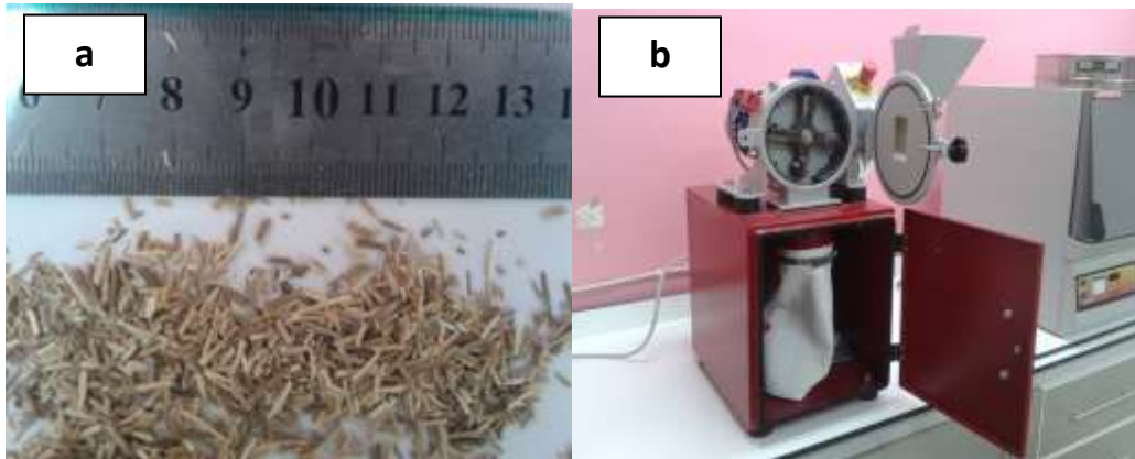
Plate 1: (a) The investigated date palm fibers and (b) Hammer mill apparatus.
