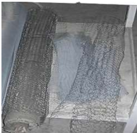
Plate 1: Galvanized hexagonal steel wire mesh.
