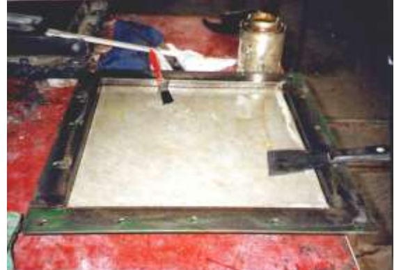
Plate (4): Furnishing and oiling light gauge base of the form.
