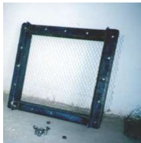
Plate 1: Galvanized hexagonal steel wire mesh.
