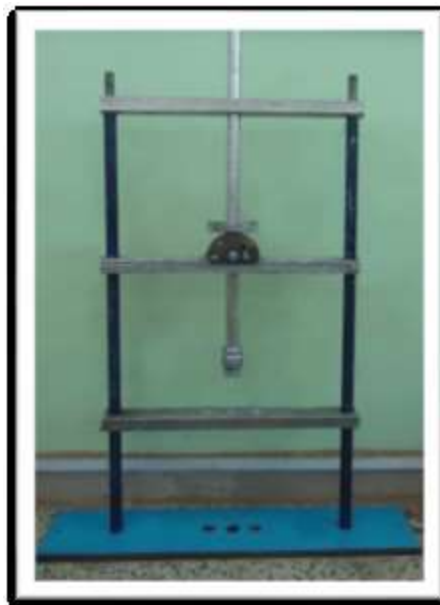
Plate (2): Piles hammer device.
