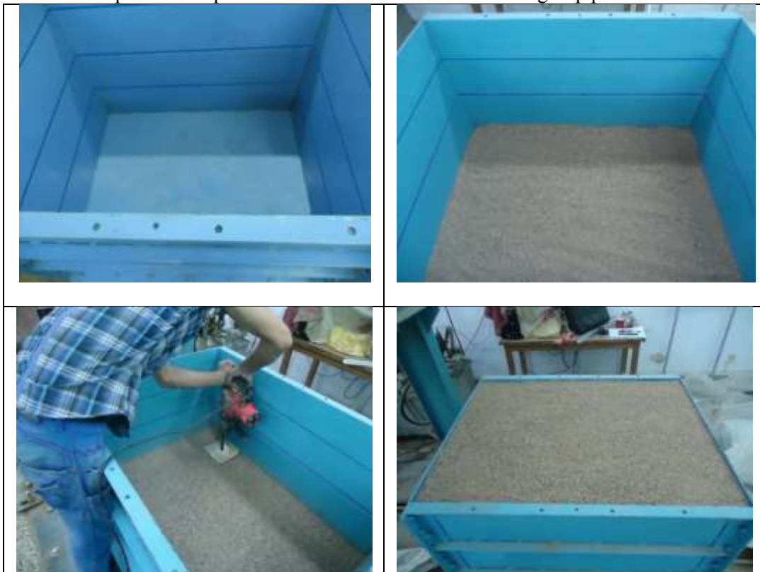
Figure (3): represents the sand deposit preparation.
