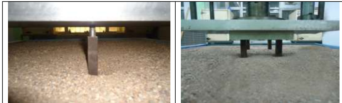
Figure (4): Installation of model piles.
