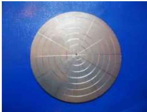
Figure (5) The blank with grids, by using mechanical grid marker
