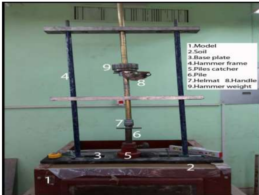
Figure (1): Model and Pile driving hammer device.
