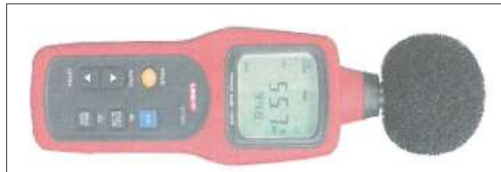
(1): The device used for measuring noise level (Sound Pressure Level Meter Type 2 UT 351)
