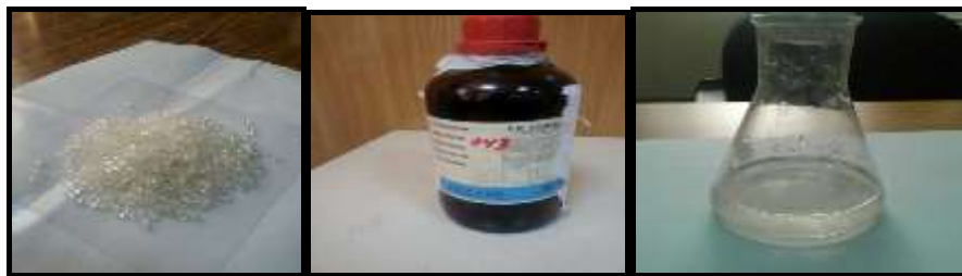
Figure (1): PC pellet and its solvent (a) PC pellet (b) Chloroform (c) PC pellets after dissolving.
