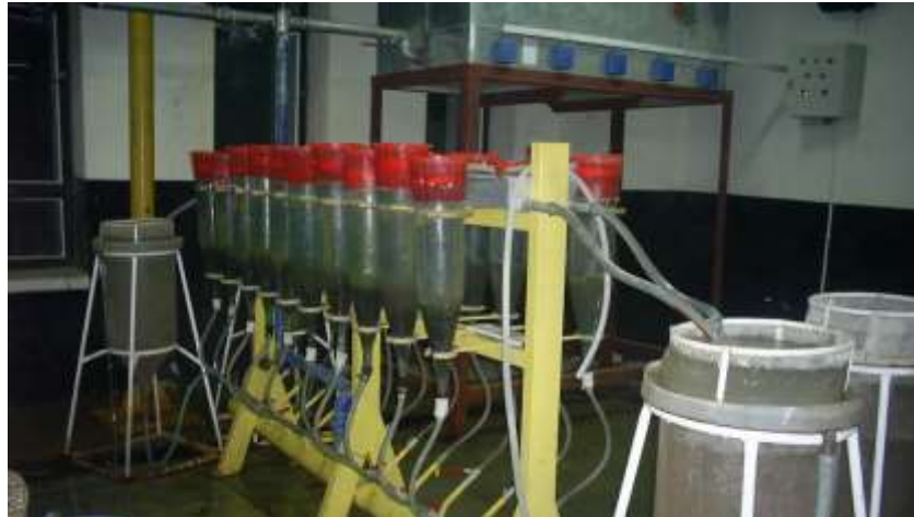
Picture (1) Semi-circulatory system in Alwahda fish hatchery which used in this study .
