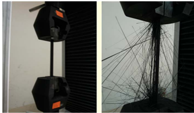
a)The specimen before test b) The specimen after Failure Figure ( 1): Tensile test of CFRP laminate
