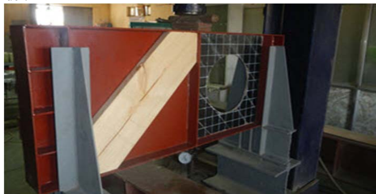
Figure (4): Test setup for plate girder specimen
