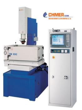
Figure(2)EDM machine used for the experimentation
