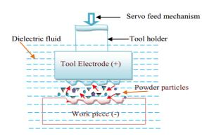
Figure (1) the principle of PMEDM [5]
