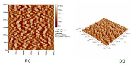
Figure (3) 3<sub>a</sub> and 3<sub>b</sub>: AFM image of Ag NPs in two dimensions and three dimensions respectively
