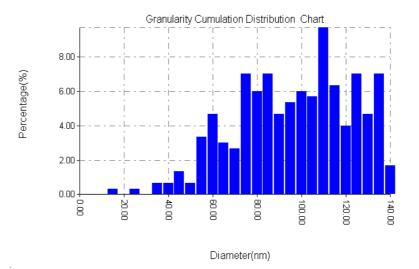
Figure (2):The histogram of Ag NPs size.
