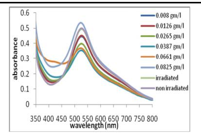
Figure (4)b : DPPH absorbance at 526 nm after irradiation
