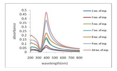
Figure(1) UV-VIS absorption spectra of silver nanoparticles functions of its concentration
