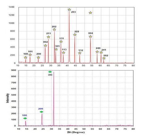
Figure (3): XRD of hydroxyapatite prepared using chemical method. 1156
