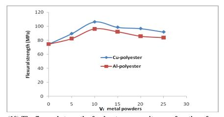
Figure (10) The flexural strength of polyester composites as a function of a metal powders content in composites.
