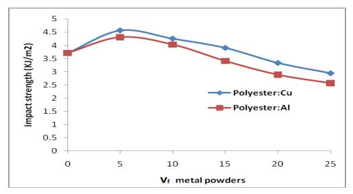
Figure (12) Impact strength of polyester composites as a function of metal powders content in composites.
