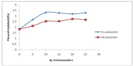
Figure (11) flexural modulus of polyester composites as a function of metal powders content in composite.
