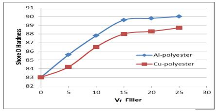
Figure (14) Shore D hardness of polymer composites as function of of metal powder content.
