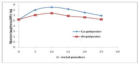
Figure (13) Fracture toughness of polyester composites as a function of metal powders content in composite.
