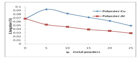
Figure (9) The elongation at break of polyester composites as a function of metal powder (Cu and Al) content in composites
