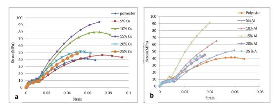
Figure(5) The stress-strain curves of unsaturated polyester composites as function of particles content in the composite (a) of Cu and (b) of Al.
