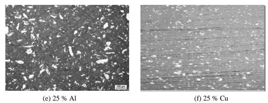
Figure (15) Optical photographs for unsaturated polyester reinforced with Aluminum particles (a, c and e) and copper particles (b, d and f) at different ratios (5%, !5 % and 25%) respectively (200 X).
