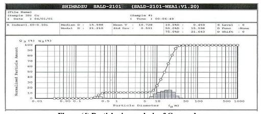
Figure (4) Particle size analysis of Cu powder.
