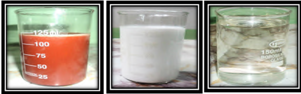
Figure(1) Show nanofluids for Cu + Dw , TiO 2 + Dw and Dw
