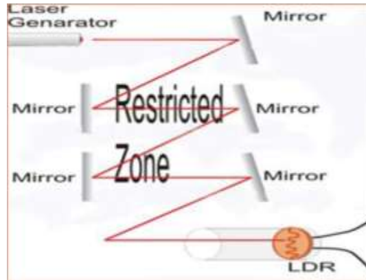
Figure (1): Laser Fence System
